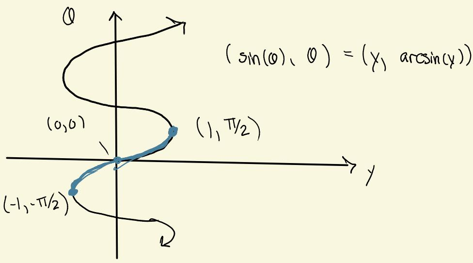
$$\Rightarrow \boxed{\text{dom}(\arcsin)} = \text{rng}(\overline{\sin}) = [-1, 1] \quad \checkmark$$
